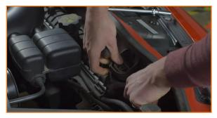
2. Transfer the bushing on the upper radiator support to the catch can bracket.
