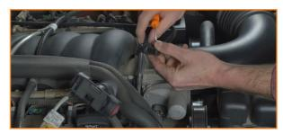
6. Connect the longer hose to the back of the engine. Run the hose up to the catch can bracket.
