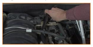
7. Connect the smaller hose to the open port at the front of the engine.
